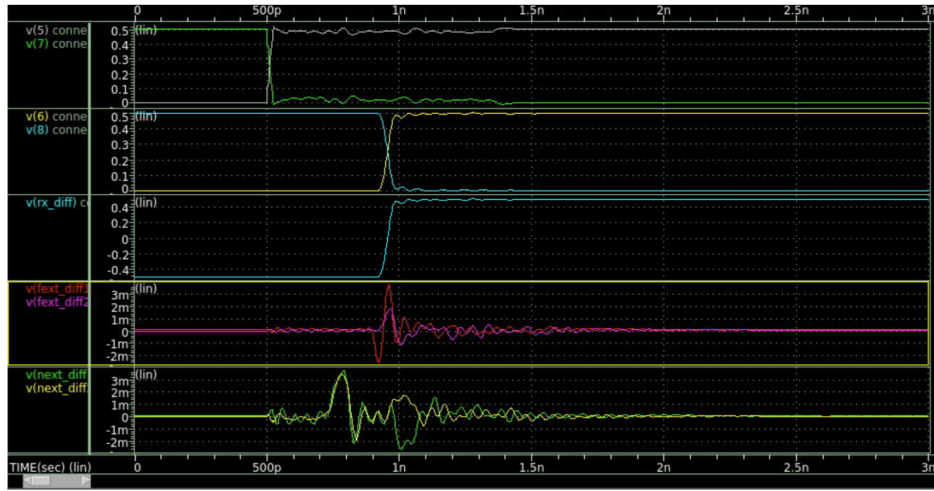
Figure 17: Orthogonal midplane connector crosstalk analysis.
